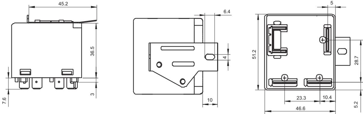
Remark: In case of no tolerance shown in outline dimension: outline dimension  $\leq 1$ mm, tolerance should be  $\pm 0.2$ mm; outline dimension  $> 1$ mm and  $\leq 5$ mm, tolerance should be  $\pm 0.3$ mm; outline dimension  $> 5$ mm, tolerance should be  $\pm 0.4$ mm.
