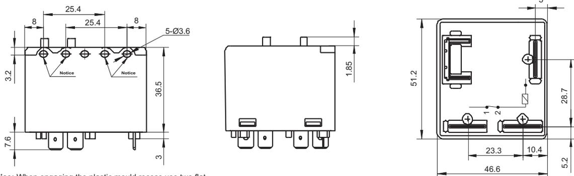
**Notice:** When engaging the plastic mould recess, use two flat head, self tapping screw, size 4.2mm, 9.5mm long.
