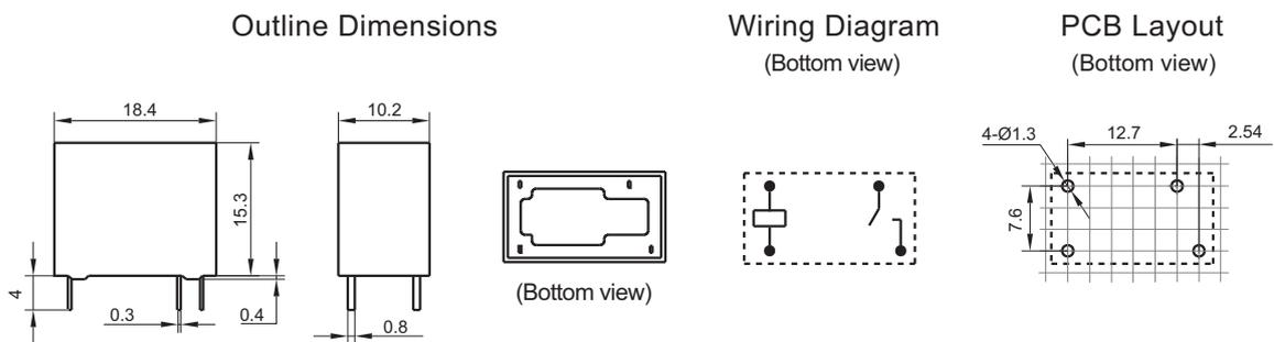
Remark: 1) In case of no tolerance shown in outline dimension: outline dimension  $\leq 1$ mm, tolerance should be  $\pm 0.2$ mm; outline dimension  $> 1$ mm and  $\leq 5$ mm, tolerance should be  $\pm 0.3$ mm; outline dimension  $> 5$ mm, tolerance should be  $\pm 0.4$ mm.
